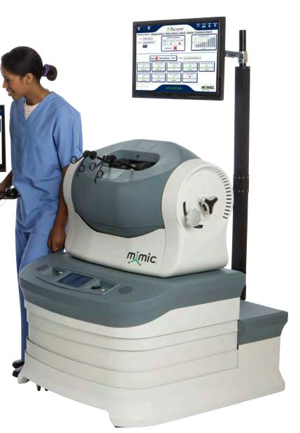
The **dV-Trainer** is a da Vinci® Surgeon's Console emulator that recreates the look and feel of operating with the da Vinci® robot. Because the dV-Trainer allows for training outside of the operating room, utilization is typically much greater than with the Skills Simulator (a.k.a. "the Backpack") due to greater accessibility. The dV-Trainer features a stereoscope, grips, foot pedals, and force effects that mimic the da Vinci® Surgeon's Console.
